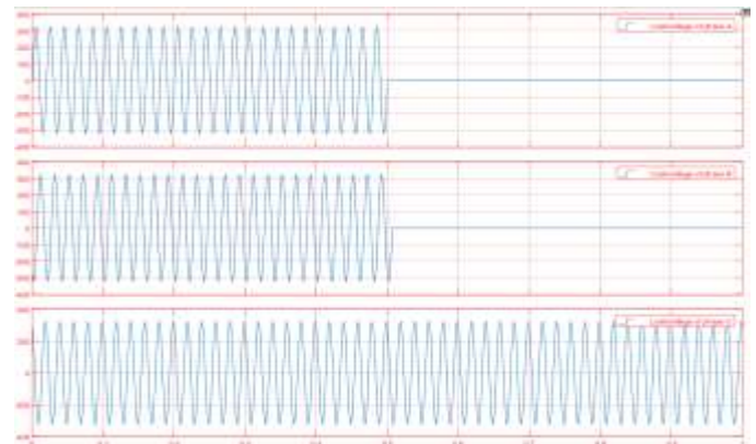
Fig 5.5 Phase A, phase B fault without STATCOM
